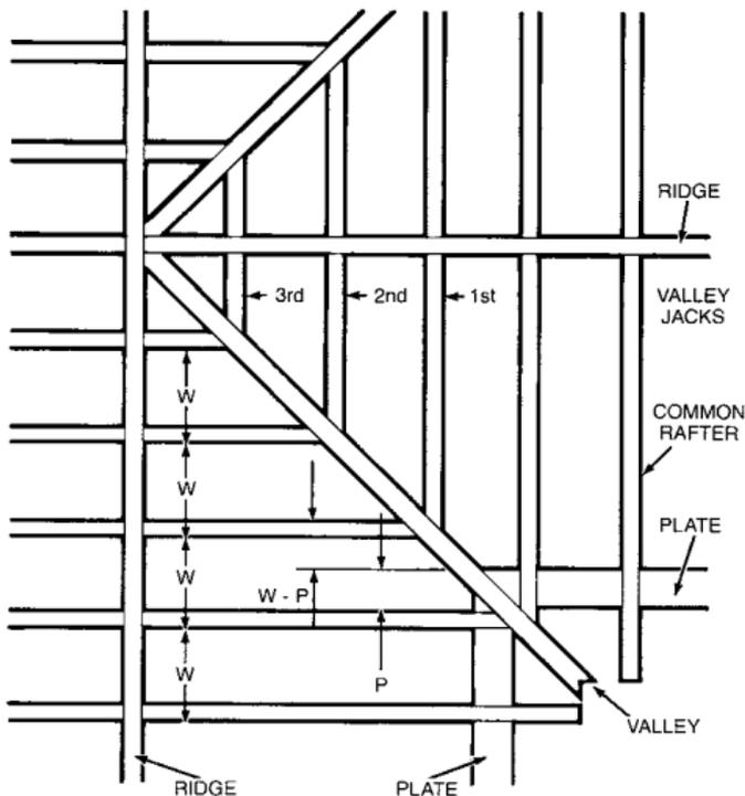
**FIG. 15 Top View of Valley Jack Rafter Spacing.**
