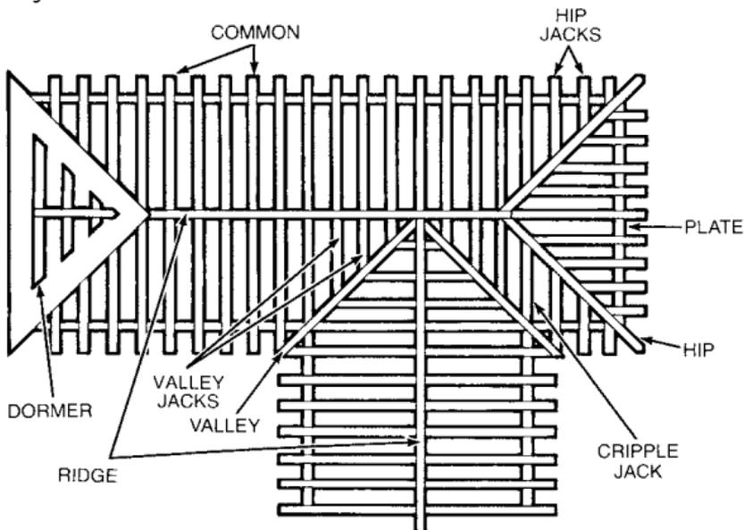
FIG. 8 Top View Rafter Definition.
