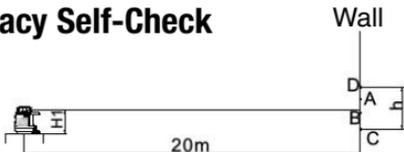
1. Set up the instrument on a table 65 ft. (20m) away from an indoor wall, with one of the X-axes facing the wall as indicated by the "X" marked on the top of the unit.
