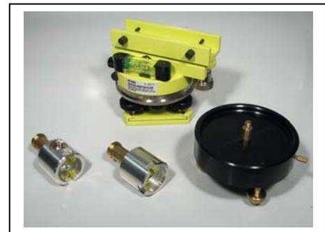
The AP90C Beam Bender adapts to the GL100 MX Laser Precision Level and creates two laser beams that are exactly 90 degrees apart. This is used for quick layouts, exact positioning of reference points and vertical plumbing. The AP180C Beam Spreader creates a line useful for layouts, marking and broad area leveling.
