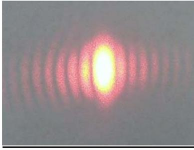
The laser beam center is positioned 1/2 inch from the bottom of the level. This means that a half inch needs to be subtracted from the center spot of the laser dot to reference the actual bottom of the level.
