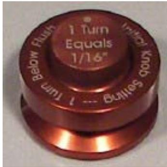
Initial knob setting is to extend the magnet bottom outward from the target bottom by one full turn (1/16") so target groove center is elevated 0.312" off magnet bottom. Adjust knob up or down from this.
