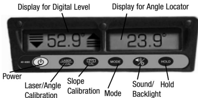
The instrument has six operating keys with their functions below:
