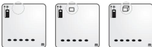
Follow flashing line instructions on screen to measure length, width & height. Press and release
