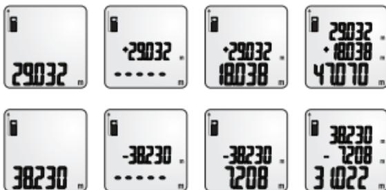
This laser distance measure has the capability to add or subtract area, volume or indirect measurement calculations. For example, if you need the square footage of four rooms this instrument will allow you to add each area calculation together to sum the dimensions of the four rooms. The same holds true for volume or indirect measurement modes. Please see each respective measurement section for the step-by-step instructions.
