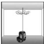
Plumb reference for lamp installation
