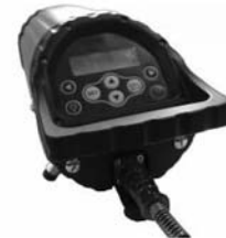
Charging the battery pack with rechargeable battery pack in laser
