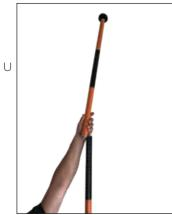
5. You can extend the overall height of the laser pole by twisting the black connector piece on the end of the spring loaded pole (V). Rotate the black connector piece 1/8" counterclockwise to unlock, extend and lock into position (W) by turning clockwise. Note, the overall pole height should be 1/4" - 1/2" longer than the ceiling height to allow for sufficient spring loaded pressure.
