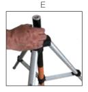
3. Use leveling vial to level tripod and make adjustment to each leg as needed (F).
