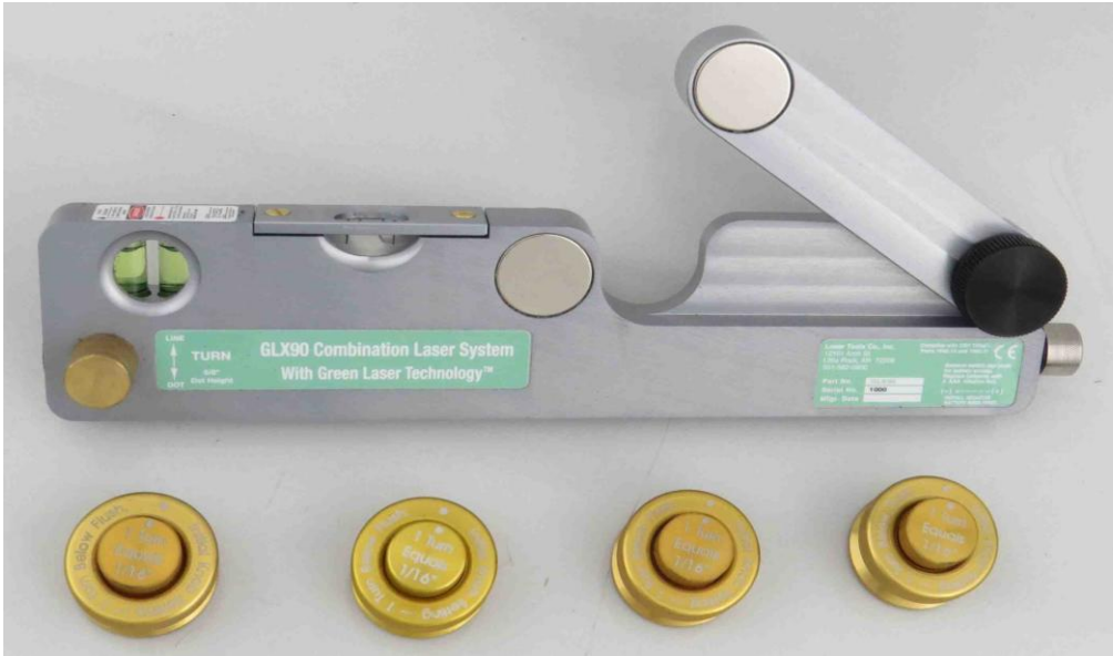
Plumb and Level Vials Front Side Magnets Offset Swing Arm Turret Product Identification Label Battery End Cap Switch Four Magnetic Targets
