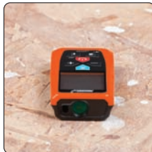
Cal3: Rotate 180°, LCD towards you.
