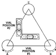
Keep about half the length engaged. When the bubble is centered in position #1, turn the instrument and observe the vial in position #2. Now center the bubble in position #2 using only screw C. The instrument should now be leveled, but to be certain, double-check. Rotate the instrument  $180^\circ$  so the vial is reversed. If the bubble will not center when reversed, follow adjustment procedure outlined under "Bubble Adjustments."
