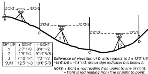
The difference of elevation between D and A is found by taking the difference between the sum of the plus sights and the sum of the minus sights. If the sum of the plus sights is larger, the final point is higher than the starting point. If the sum of the minus sights is larger, the final point is lower than the starting point.
