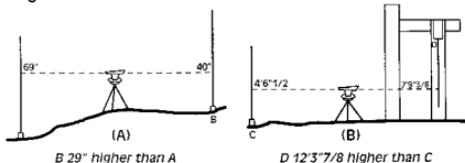
A line of sight 69 inches above A and 40 inches above B is shown above. Therefore, B is higher than A by 29 inches.
