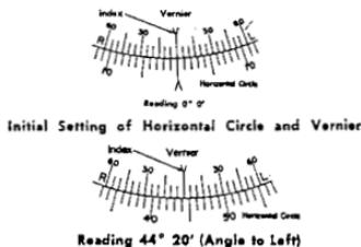
In the illustration above, the index has passed the 44 degree line but has not gone as far as the 45 degree line. In this case, the third vernier line from the index is lined up with one of the lines on the circle. Since each vernier line represents 15 minutes add 45 minutes to the 44 degree reading (3 times 15 minutes equals 45 minutes). Therefore our exact reading is 44 degrees, 45 minutes ( $44^{\circ}45'$ ).
