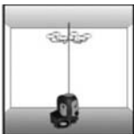
Plumb reference for lamp installation
