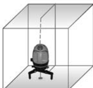
Front vertical and plumb point
