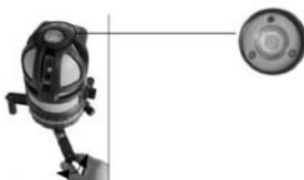
Adjusting the bubble
