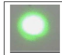
The laser beam center is positioned 1/2 inch from the bottom of the level. This means that a half inch needs to be subtracted from the center spot of the laser dot to reference the actual bottom of the level.
