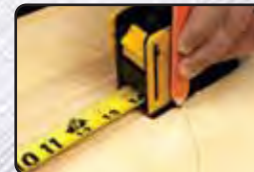
Marking Radius with Nail in 1" Grommet
