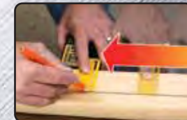
Marking Along a Parallel Edge
