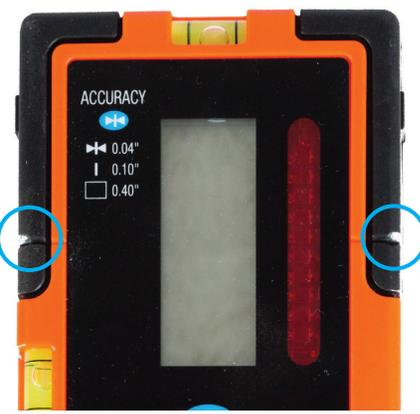
**IF NOT USING A GRADE ROD:** Read grade position using the grade position indicators on the housing of the laser detector (shown with the blue circles in the image to the left). For your convenience, an indent in the housing will help locate a pencil, marker or other marking tool so that you can mark the grade position directly on your work surface.
