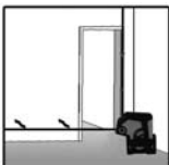
Reference for door frame installation
