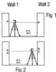
**Note:** This accuracy checking method doubles the error. For example, if the difference between Point A and Point D is 1/4" at 25', your laser is accurate to 1/8" at 25'.
