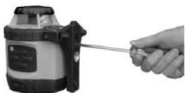
Calibration of Y-direction
