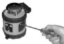
Calibration of X-direction
