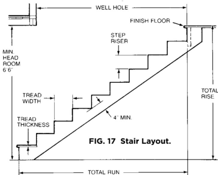
**NOTE 1** Before starting your layout, check local and state codes for tread width, length and step rise requirements. Many states have stairway construction regulations.
