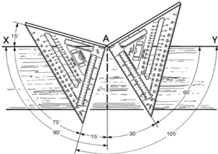
SQUARE SHOWN IN 2 DIFFERENT POSITIONS WITH THE RESULTING ANGLES BEING FOUND BY PIVOTING SQUARE AT POINT (A) ON LINE X-Y.
