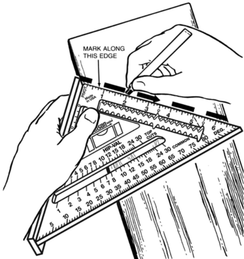
DRAWING SHOWS SQUARE IN POSITION FOR MARKING TOP PLUMB CUT OF A COMMON RAFTER WITH AN 8" RISE, ALSO SHOWING A  $33\frac{3}{4}^{\circ}$  ANGLE.
