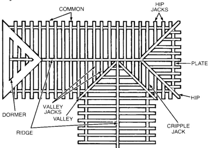
FIG. 8 Top View Rafter Definition.
